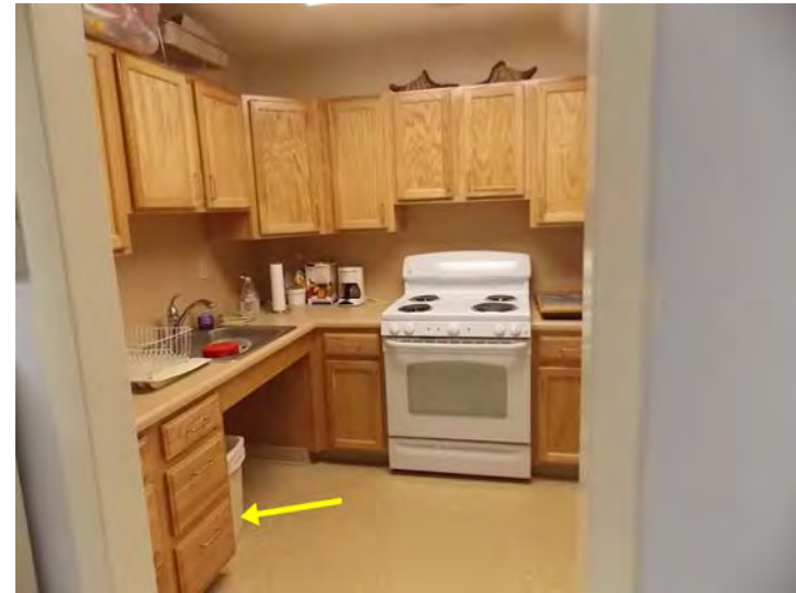
This is the community kitchen. This space should be modified to include a 30-inch work surface that has adequate knee space (possibly by having a removable base cabinet –see arrow)
